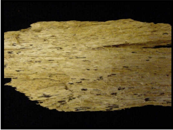
~ Caption: Annosus root rot decayed wood with black flecks ~ Photo by: B.M. Johnson
